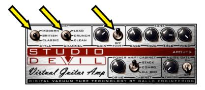
The **STYLE** switch, **CHANNEL** switch, and **BOOST** switch all work together to select the type of amplifier you're looking for. Here's how they work:
