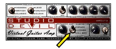
Without a guitar speaker cabinet, guitar distortion would sound thin and harsh. The "cabinet" switch allows you to select a basic cabinet modeling filter to get the effect of hooking your amp up to a real guitar cabinet. There are 3 settings to choose from:
