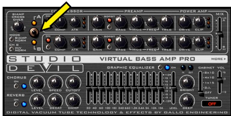
The CHANNEL SELECT A/B switch has a few uses. First, it can be used as a typical channel switch, letting you toggle between two distinct sounds, like you would in a live situation. Second, you can use it as an A/B test, to hear the differences between two different sounds when making fine adjustments. You can also use it to help you hear the best spot to set the BIAMP CROSSOVER frequency knob when operating in BIAMP mode. The possibilities are endless!
