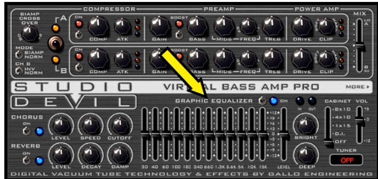
**EQ SLIDERS:** Each of the graphic EQ's twelve sliders (starting from the left) lets you adjust the boost or cut for frequencies within a certain band. Slide the handle up for more boost, or slide it down for less. Going from left to right, the frequency bands go from bass (lows) to treble (highs). The frequencies for each band are specifically chosen to work well with bass guitar and to give you lots of control over your sound.
