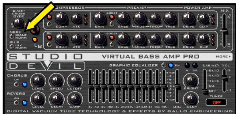
**BIAMP CROSSOVER KNOB:** This knob only works in BIAMP mode (see MODE SWITCH above). This control lets you set the crossover frequency, which is the point where the BIAMP crossover splits your bass guitar input signal into lows and highs. This knob selects a frequency crossover point from the range 40Hz to 8kHz. When in BIAMP mode, the frequencies below this knob setting are sent to CHANNEL A, and the frequencies above this setting are sent to CHANNEL B.
