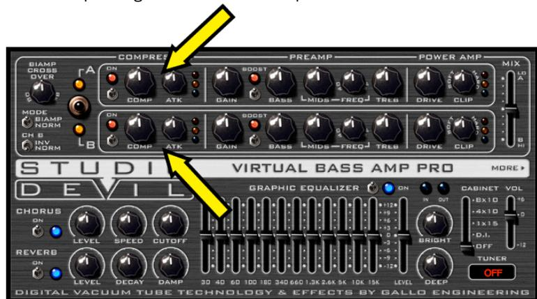
**AMOUNT KNOB:** This knob controls how much compression and sustain you get by setting the peak gain boost of the compressor. Turn this knob to the right for more sustain and boost, or to the left for less gain and more
